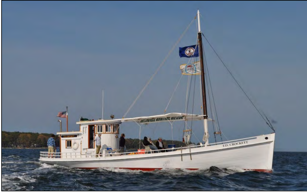
^The NRHP-listed F.D. Crockett (DHR ID #059-5013) is a log-hulled deck boat constructed in 1924 by Alexander Gaines, one of the last traditional log boat builders in the Middlesex County area, and is representative of Tidewater region's tradition of log boat construction as well as the Chesapeake Bay buyboat form. (VLR Online)
